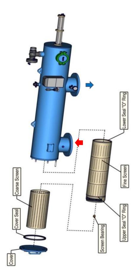
Figure 7: Fine Screen Assembly Removal & Installation
