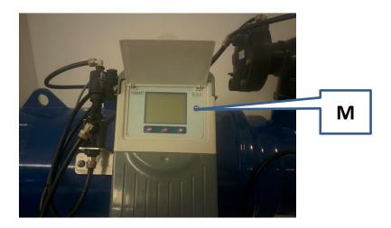
Figure 3: Battery Removal & Installation
